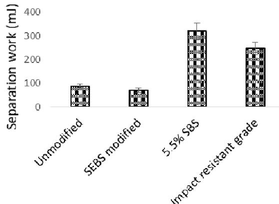
Fig.5. Total work or energy required for sample separation.
