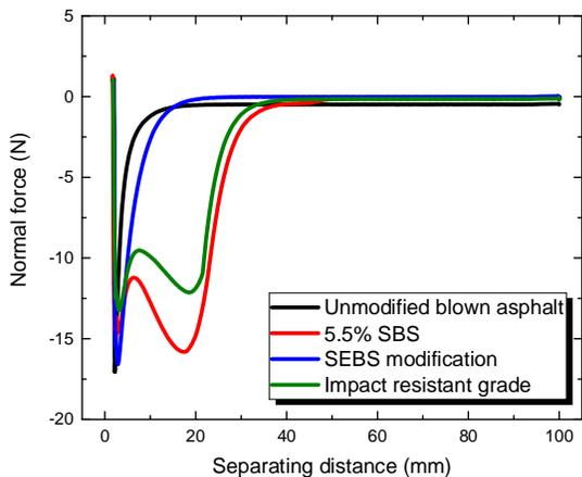
Fig. 4 Normal force vs. separating distance after 1N contact force for 10 s at 50 °C.
