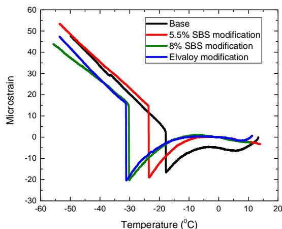
Fig. 3. Strain change with temperature during cooling for base asphalt and SBS, Elvaloy modifications (4 runs for each sample were tested and one of them is randomly selected here)
