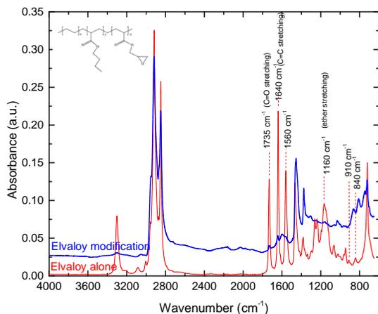
Fig.2 FTIR-ATR spectra of Elvaloy itself and Elvaloy modified asphalt.
