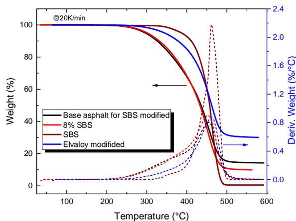
Fig.1. TGA curves and its derivative curves at 20K/min under nitrogen of SBS, base asphalt, SBS modification and Elvaloy modification.
